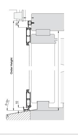
Sliding Unit ST3/24 double-sash with 1 & 2 fold track
