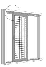
The spring force of the sliding sash guide **5** can be adjusted if required: To do this, loosen screw with the provided Allen key **4**, adjust spring force and tighten screw again **6**.
