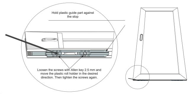
The location of the set screw with respect to " + " and " - " shows the current height position of the roller.
