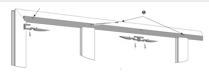
Position drilling jig 164851 at marking done in step 2. Predrill through the two outside holes with 2.2mm drill bit. Then mark centre position. Position drill jig 6mm to the left and right of centre position and predrill through the two outside holes. Attach stoppers with LK2.9x16
