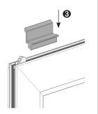
**⑤** Position top guide rail according to markings. Predrill window frame through predrilled holes in guide rail.
