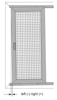
By moving the plastic roll holder in the (+) direction, the sliding sash on this side moves upwards by 1 mm.
