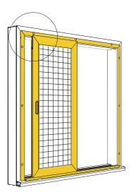
The spring force of the sliding sash guide **⑤** can be adjusted if required: To do this, loosen screw with the provided Allen key **④**, adjust spring force and tighten screw again **⑥**.
