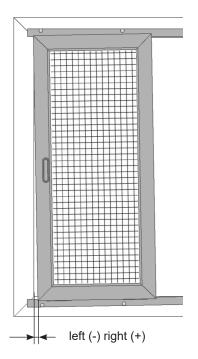
By moving the plastic roll holder in the ( + ) direction, the sliding sash on this side moves upwards by 1 mm.
